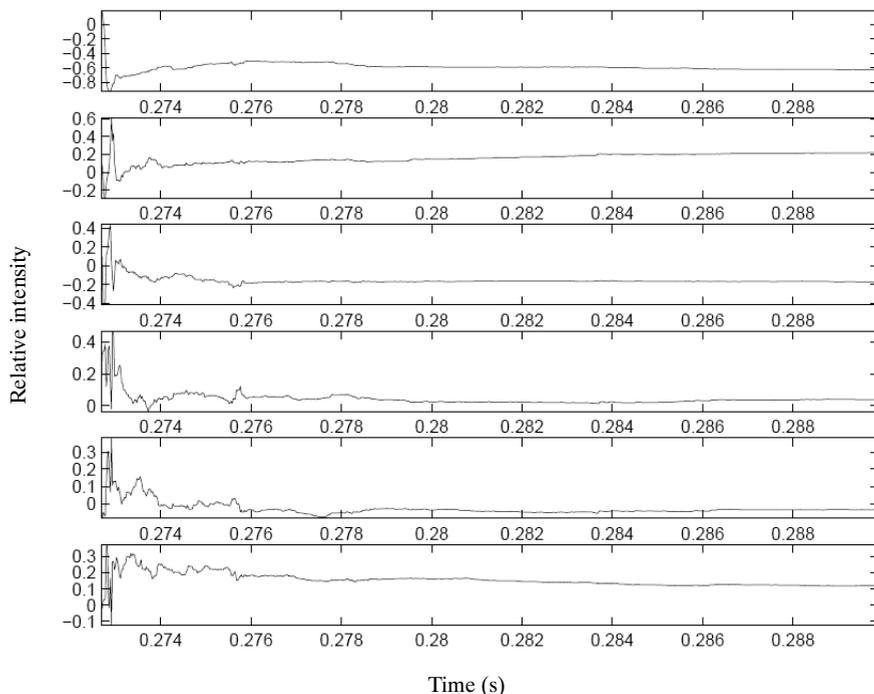
Fig. 3. Changes of the time-domain structure (Shur coefficients) in the selected six cells of the parametrization filter (relative intensity = maximal sound pressure/temporary sound pressure).
