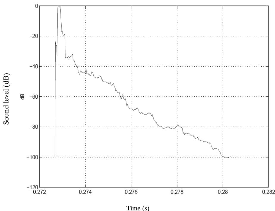
Fig. 5. Changes in transient acoustic power. Notes. In this graph 0 dB = 138, 2 dB of sound pressure; weapon: Margolin (Izhevsky Mekhanichesky Zavod, USSR); 25-m shooting range.
