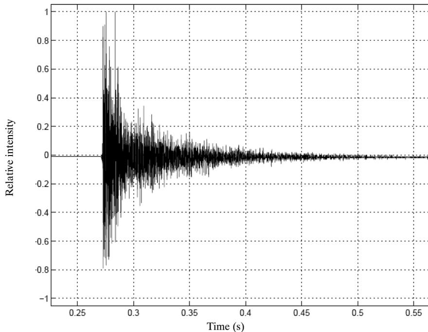
Fig. 2. Time history of an acoustic signal (relative intensity = maximal sound pressure/temporary sound pressure). Notes. Weapon: Margolin (Izhevsky Mekhanichesky Zavod, USSR); 25-m shooting range
