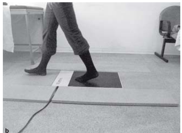
Fig. 1 a and b. Gait analysis with the use of Pressure Distribution Measurement System (PDM-S) force-plate
